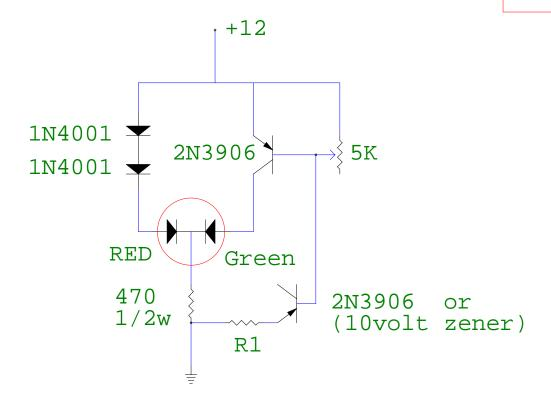
For about 1 volt range (from full red only to full green only), make R1 10K. For about .5 volt range, make R1 4.7K. I prefer the 1 volt range, with full red at about 12 volts (full green by about 13 volts).
